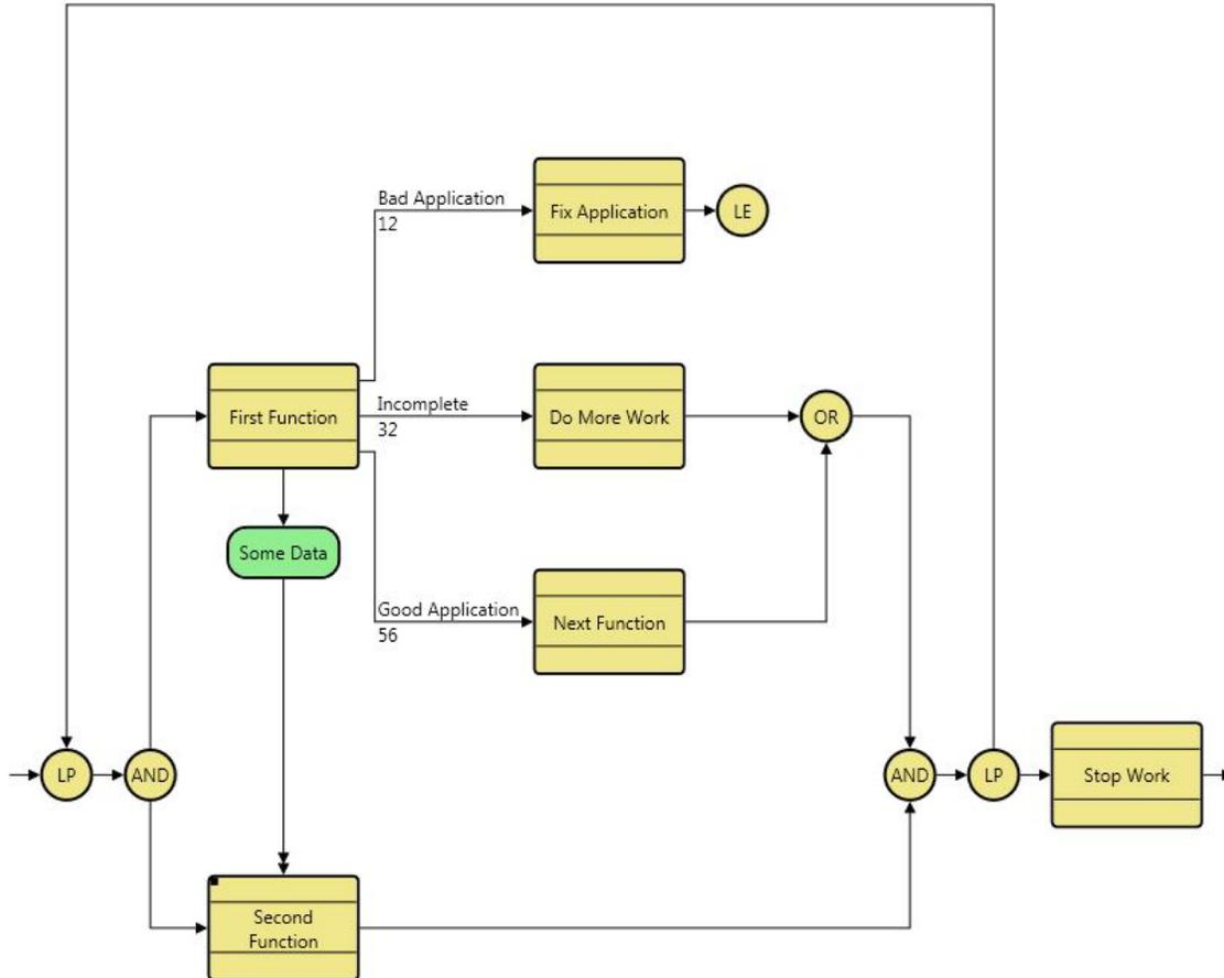
Figure 43 EFFBD with Loop and Loop Exit
