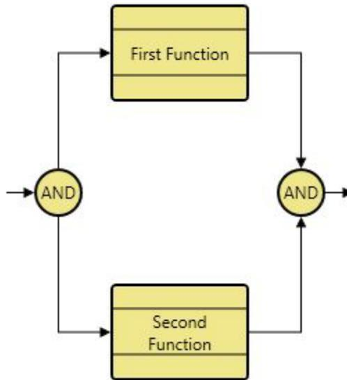
Figure 26 Parallel Construct
